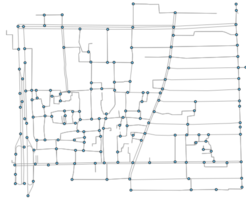
Fig. 4: Node diagram for candidate RSU locations. The circles are candidate locations of RSUs and solid lines are roads.
